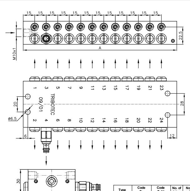
In the case of plugging of outlet grease (double dose) is necessary for the correct operation of the distribution to remove the screw -position 3.
